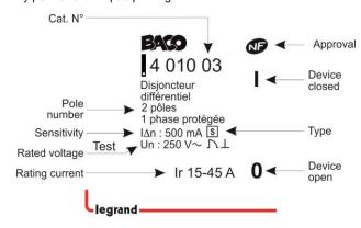
Rated voltage: . 250 V~ / 50 Hz between phase and neutral . 440 V~ / 50 Hz between phases
